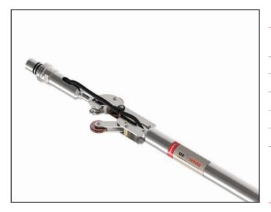
The IPI-X is an Automatic Magnetic Extensometer combined with an In-Place Inclinometer which can be used typically to measure vertical and horizontal displacement in embankments, dam foundations, deep foundations and around tunnels and diaphragm walls.
