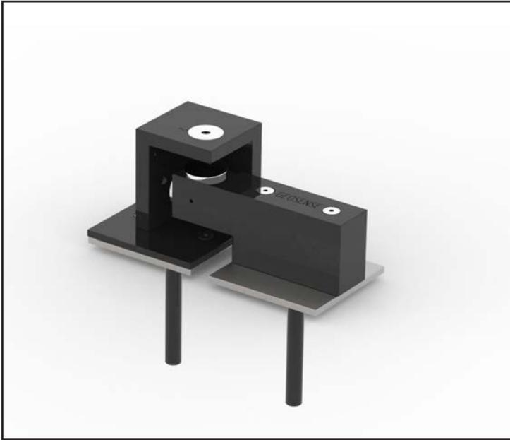
Geosense® 3D crack meters are designed to monitor three way displacement (X, Y and Z) across joints or cracks between adjoining concrete and rock structures.
