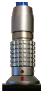
Figure 9 - Lemo Connector to GK-404
