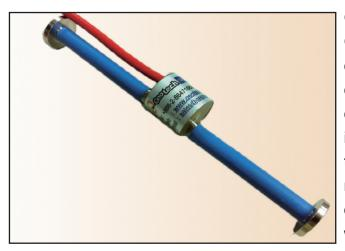
GT-VG-4200 Concrete Embedment Strain Gage is usually used for monitoring the change of strain in either reinforced concrete or mass concrete structure during the construction period. Inside the gage there is a length of string wire which is fixed and tensioned between two steel blocks. Deformation of concrete structure changes the distance between two steel blocks, thus it will alter the tension in string wire.
