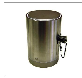
The Geosense® SGLC 7050 series load cell consists of a solid cylinder of high strength stainless steel with a series of electrical resistance strain gauges connected around the periphery as a Wheatstone Bridge that compensates for unevenly distributed loads and provides a single mV/V signal output.
