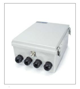
A four-conductor cable (with shield) supplies power and control signals from the datalogger to the GT10-16. The GT10-16 requires one datalogger control port for enable (reset terminal), and a second control port to advance through the channels (clock terminal). Either the datalogger's power supply or a separate 12 V supply is used to power the multiplexer. Geotech Science Co., Ltd. offers the cable to connect the GT10-16 to the datalogger's power terminals and control ports.
