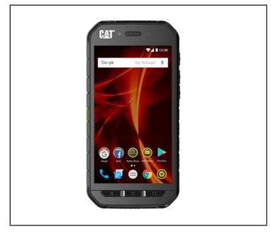
The CAT® S41 smartphone is used as a handheld readout to configure and collect data using a purpose-designed app.
