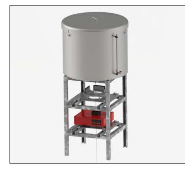
Geosense® HPS-3500 (Hanging) and IPS-3000 (Inverted) Pendulums are used to measure the tilt or rotation by measuring the relative internal horizontal displacement of points along a true vertical line. Each has a tensioned, stainless steel wire and the effects of the earth gravitational forces to guarantee a perfectly vertical line between a fixed point and a tensioning mechanism. Typical applications include concrete dams, bridges and high rise buildings.
