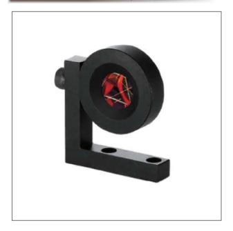
P101 circular prism is built by cutting from a solid glass cube. This creates three mutually orthogonal reflecting surfaces that reflect any light rays back towards their source. This reflector can be matched with varies total-station. (Example Leica , Sokkia and etc).
