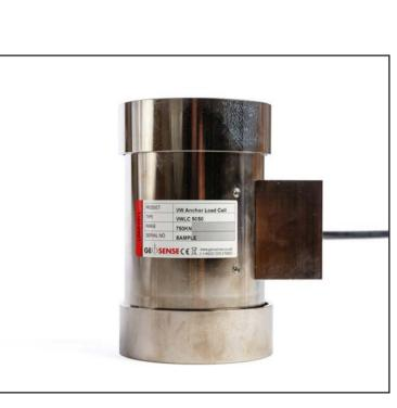
The Geosense® VWLC 5050 series of Vibrating Wire Load Cells consist of a solid cylinder of high strength steel with 3 or 5 vibrating wire strain sensors mounted parallel to the longitudinal axis arranged equidistant around the circumference which measure the compression of the cylinder under load.
