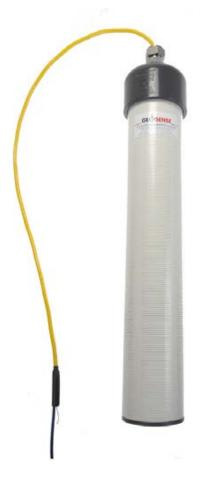
The Geosense® VWM-2000 vibrating wire precision water level monitor utilises a vented vibrating wire force transducer in combination with a cylindrical weight suspended from it to monitor water levels.
