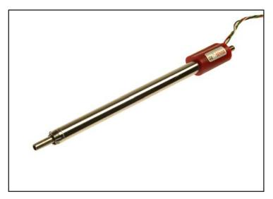
Geosense® VWDT-5000 series of vibrating wire displacement transducers cover displacement ranges up to 300mm and are fully waterproof to a minimum of IP68 (16 bar external pressure). They can be incorporated into many displacement products such as crack and joint meters, convergence meters, soil extensometers and displacement meters.
