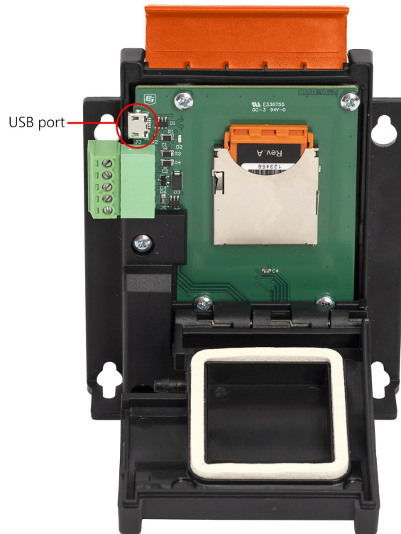
FIGURE 8-1. BaroVUE 10 with main door open
