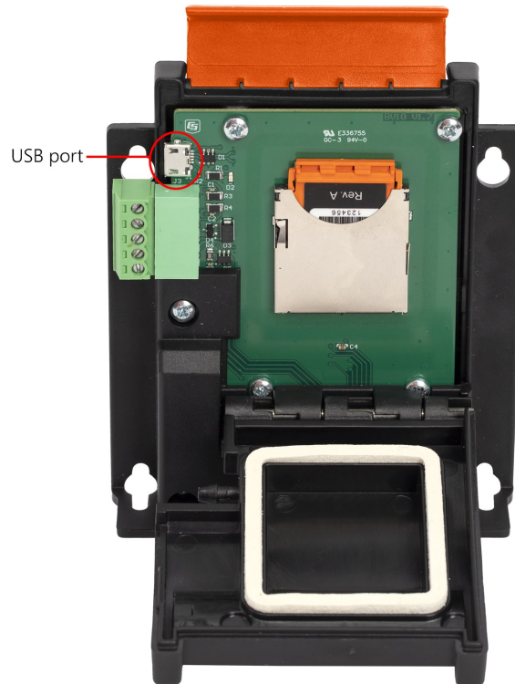
FIGURE 8-3. BaroVUE 10 with main door open
