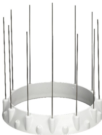
FIGURE 7-6. Spikes inserted into the plastic ring slots
