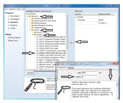
4. After selecting the sensors, click at the left of the screen on **Wiring Diagram** to see how the sensor is to be wired to the datalogger. The wiring diagram can be printed out now or after more sensors are added.
