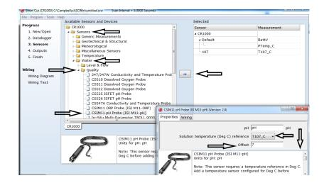
5. After selecting the sensors, click at the left of the screen on **Wiring Diagram** to see how the sensor is to be wired to the datalogger. The wiring diagram can be printed out now or after more sensors are added.
