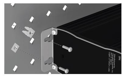
FIGURE 9-3. Enclosure backplate mounting
