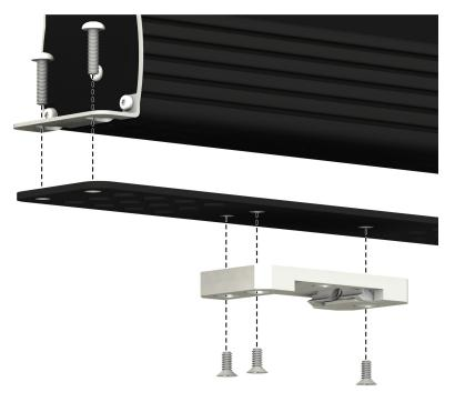
FIGURE 9-4. GRANITE DIN-Rail Mounting Kit
