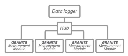
FIGURE 9-2. Multiple GRANITE Measurement Modules connected in a star topology
