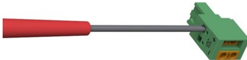
FIGURE 9-3. Opening the power connector terminals
